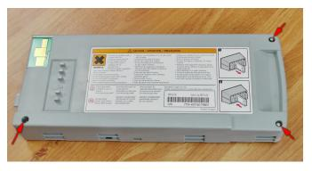
Push the tab up, slide the cover sideways and remove it.
