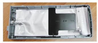
Detach the black plate. The adhesive tape will stay with the plate.
