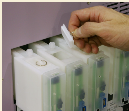
The most economical bulk system would include only the refillable cartridges that can be filled through the top opening.
